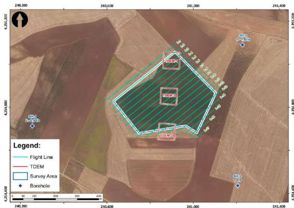
Figure 3. Flight plan made for magnetometry.
