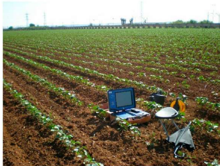
Figure 8. Terra-Tem equipment in the process of measurement.
