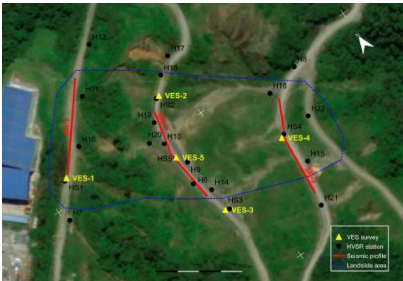
Figure 4. Situation map of surveys (noted that the north is rotated counterclockwise) and observed landslide area (blue dashed line). Black dots: HVSR surveys; yellow triangles: VES surveys; and red lines: seismic refraction and MASW profiles, both made at the same position. White crosses refer to the coordinate points (Modified from [22]).
