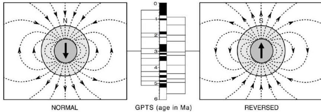
Figure 3.3 Simplified diagrams of the geomagnetic field of a geocentric axial dipole similar to the CMT dipole representing normal polarity (left) and reversed polarity (right). On the geomagnetic polarity time scale (middle column), periods of normal polarity are conventionally represented by black intervals, and periods of reversed polarity by white intervals (Langereis et al., 2010).
