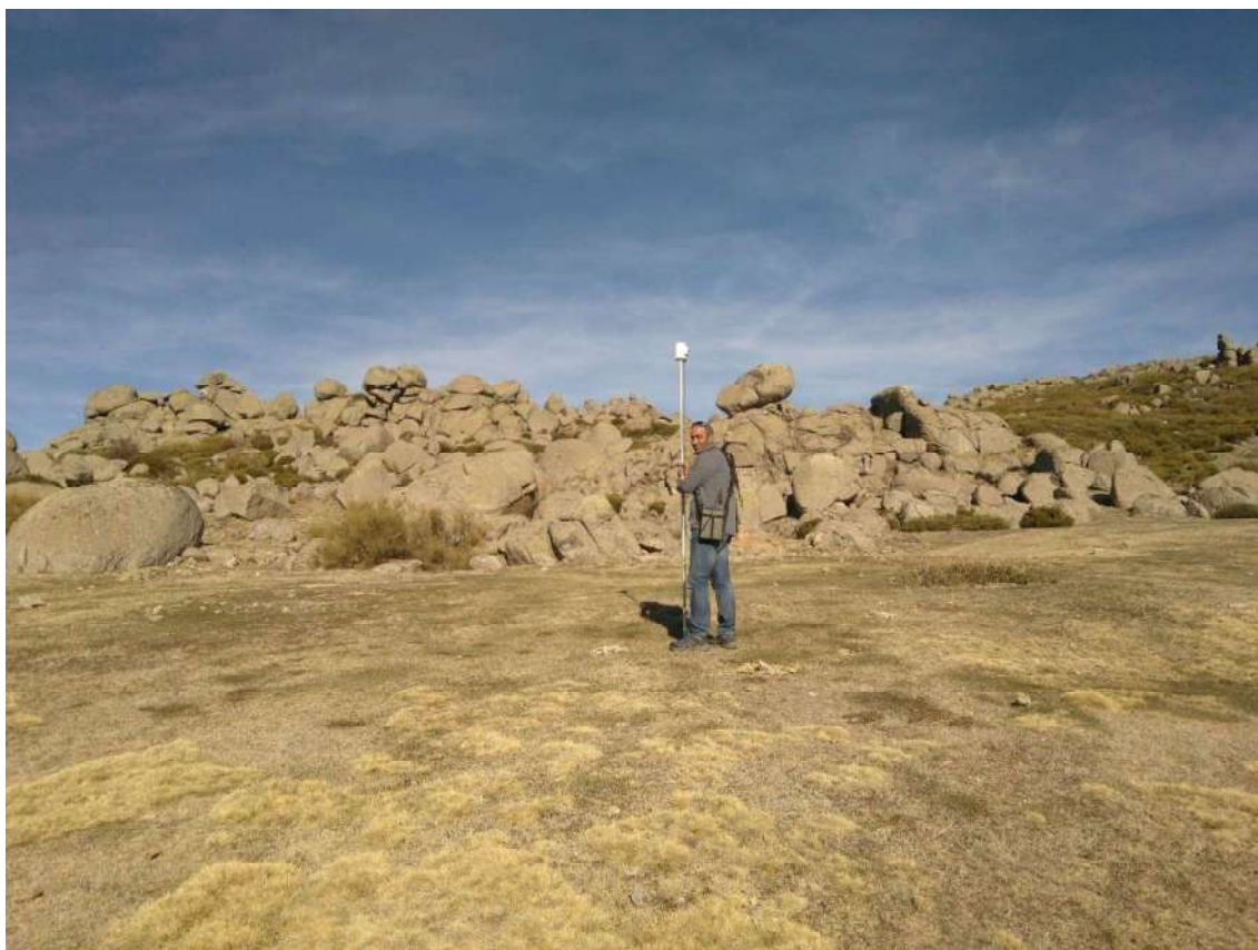
Figure 3.16 Operator holding a Geometrics G-856 proton precession magnetometer.
