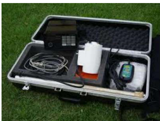
Figure 3.17 Geometrics G-856 proton precession magnetometer (left) and Garmin eTrex 10 GPS (right).
